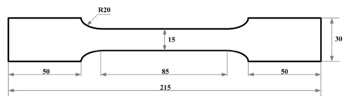
Fig. 4. The Q235 steel specimen used for investigating material properties Table 1 (unit: mm).
